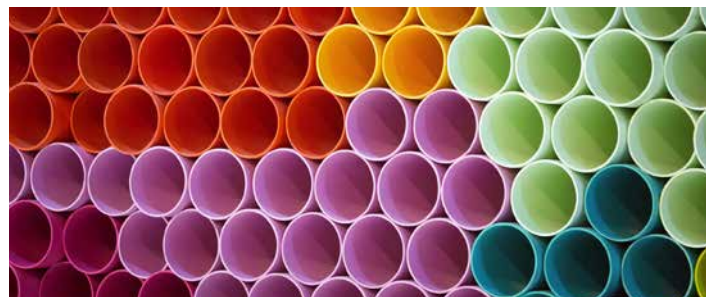
Organotins may temporarily leach from PVC pipes as they are used as a plastic stabiliser
